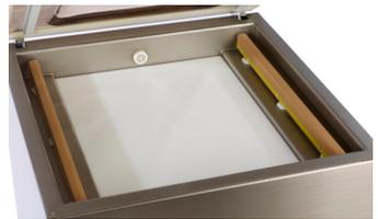
7. **Filler Plates** - Used to occupy space in the chamber. The plates allow for faster vacuum. When more space is occupied, there is less air to be removed from the chamber.
