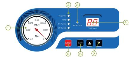
1. Vacuum Gauge: Indicates the vacuum level inside the chamber.
