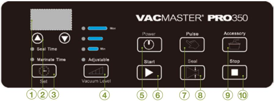
1. **Digital Display** - Displays the function settings and progress of the working cycle.
