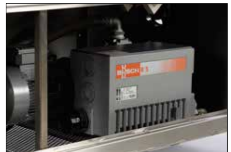
7.5 HP Busch Vacuum Pump Commercial vacuum power and a tighter seal
