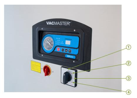
The VP680 is equipped with 3 seal bars. Using the selection switch located on the front of machine; 1 or 2 or all 3 seal bars can be made active depending on the number or size of vacuum pouches being used.
