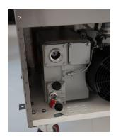
1 Remove the bottom back machine panel and the oil fill cap (black) - Locate the oil fill bolt on the back of the pump. Using your adjustable wrench, remove the oil fill bolt.
